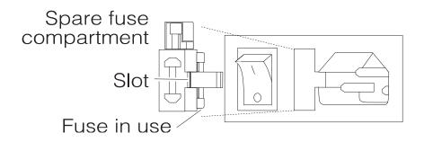
Figure 5-1: Replacing the fuse (AC power).
